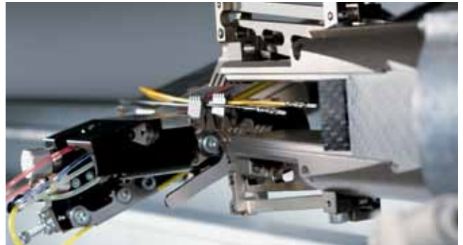
Motorized transfer bridge for gentle wire handling
