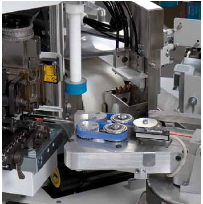
Crimp press, swivel arm, side 1 and cutting head
