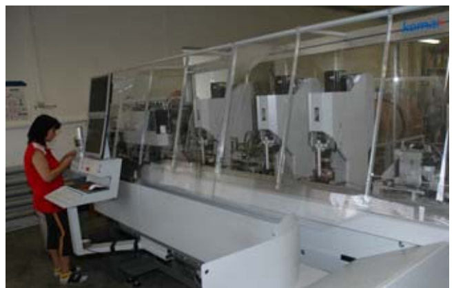
The Zeta 633/655 in action: a block loader with automatic feeding of the housings.
