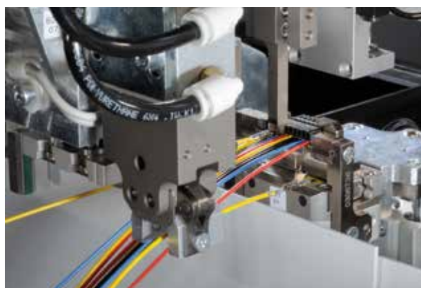
▲ Loading One-sided, double-row loading
